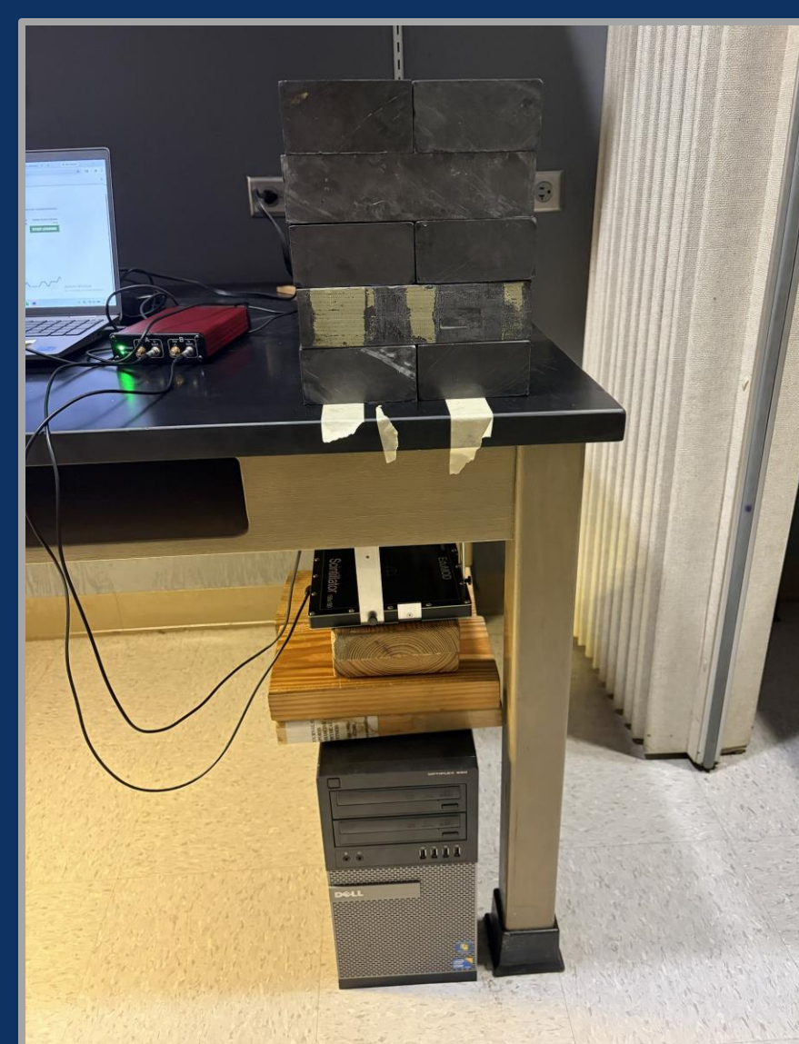
Figure 1. Experimental set-up exhibiting lead bricks above two scintillation detectors
